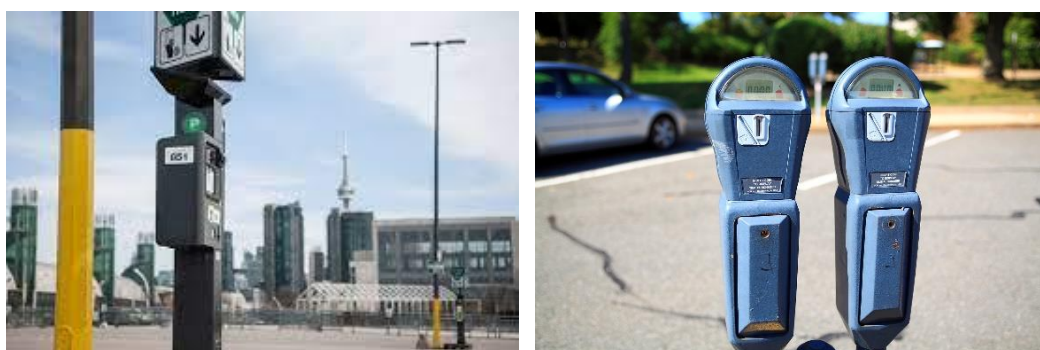
Figure 33. Sample Pictures of Single-Space-Meter (Right) and Multi-Space-Meter (Left)
